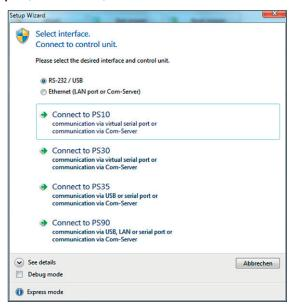
The Express Mode detects connected control unit and the required axes are configured automatically (with OWISid). The demo configuration is used for product demonstration (without hardware).
