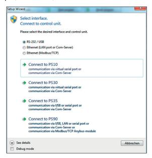
In the Expert Mode, the interface to control unit is selected, the axis configuration is load and saved from text file or in the dialog box (with or without OWISid).
