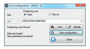
To simplify the setting you can select a suitable positioning unit from the defined program database (Find button) or from OWISid (Identify button). With the Auto-configuration button the axis configuration will be selected and saved.
